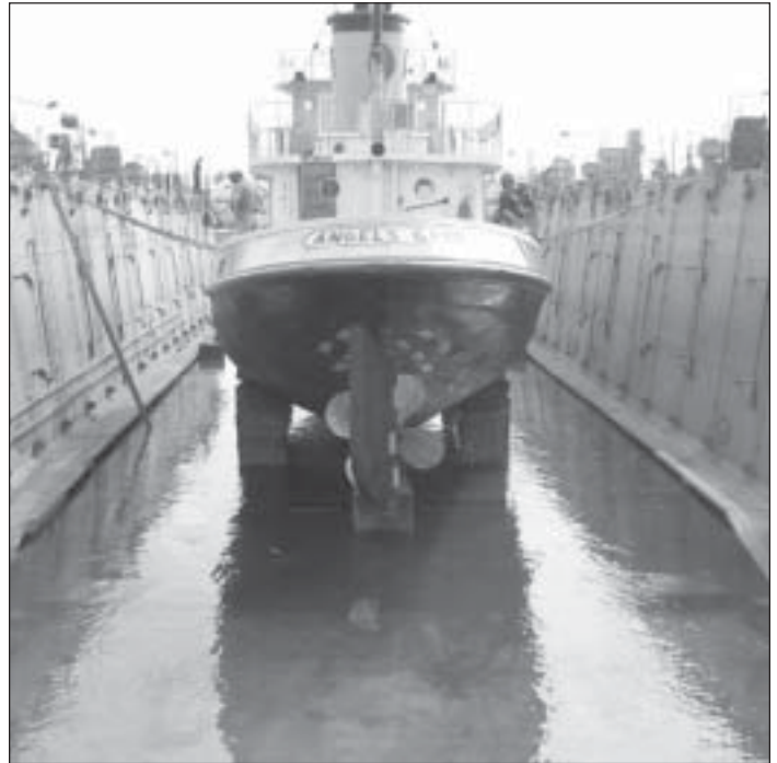
Fore and aft views of the ANGELS GATE at the Al Larson drydock show her newly-scraped and painted bottom with new zinc anodes.
