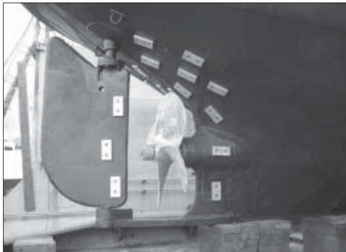
Fore and aft views of the ANGELS GATE at the Al Larson drydock show her newly-scraped and painted bottom with new zinc anodes.
